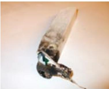
This picture shows a transformer that was removed from directly behind an open backed downlighter
